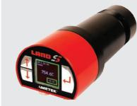
**TEMPERATURE RANGE** 200 - 1200 °C / 392 - 2192 °F An advanced non-contact infrared spot pyrometer specifically designed for continuous, highly accurate measurement of coated steel strip temperature during galvanising and galvannealing.
